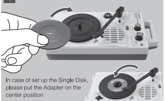
In case of set up the Single Disk, please put the Adapter on the center position
