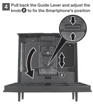
Please make sure that the Smartphone is being · fixed without sway. For some model, if being fixed too tight, the power button or volume button may be pressed by the hanger. Please o confirm the button's position before insert.
